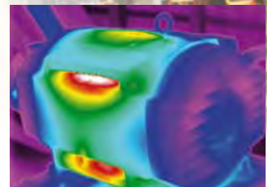
Abnormal uneven heating on motor
